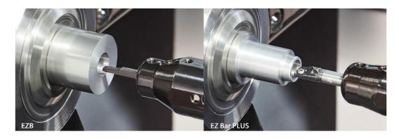
EZ Bar and EZ Bar Plus multipurpose ID turning tools for small diameter
